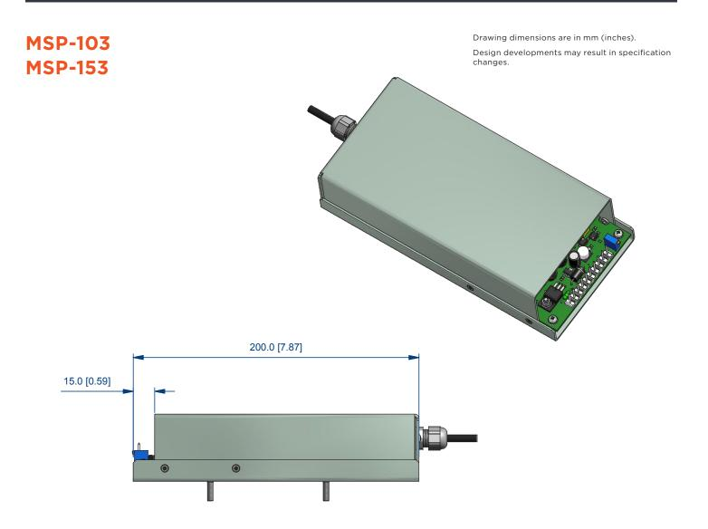
MOUNTING: 2 OFF M4 STUDS; LENGTH AND POSITION AS SHOWN DIMENSIONS mm (in)
