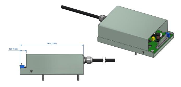
MOUNTING: 2 OFF M4 STUDS; LENGTH AND POSITION AS SHOWN DIMENSIONS mm (in)
